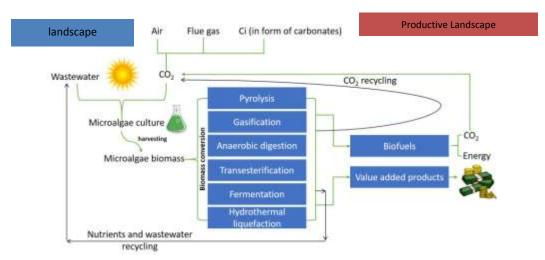
Fig. 10.The eco process in the industrial area based on algae technology (Productive landscape) Source: (Solar Gis)
